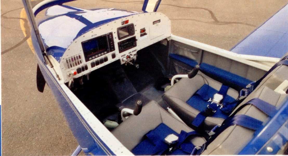
A front-mounted step allows access to the RV-12 cockpit, and the tip-up canopy is sturdy enough to handle a stiff wind (left). A Dynon display provides flight and engine information (below). A bubble canopy provides a panoramic view in flight (right).
